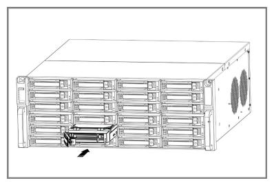
Figure 1-8 Push HDD Case into Slot
