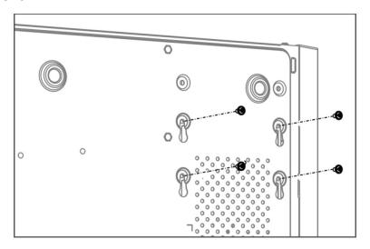
Figure 1-11 Fix HDD to Device Bottom
