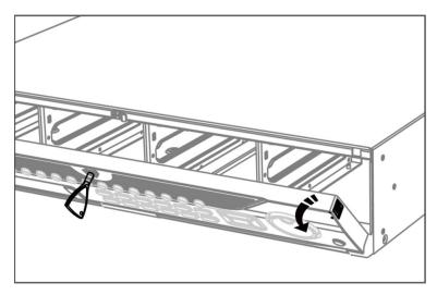
Figure 1-5 Open Front Panel
