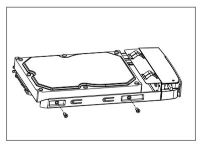
Figure 1-7 Fix HDD
