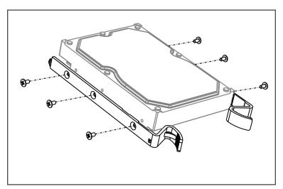
Figure 1-4 Fix Mounting Ears to HDD
