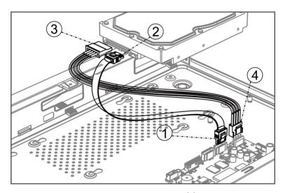
Figure 1-10 Connect Cables
