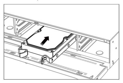
Figure 1-6 Insert HDD
